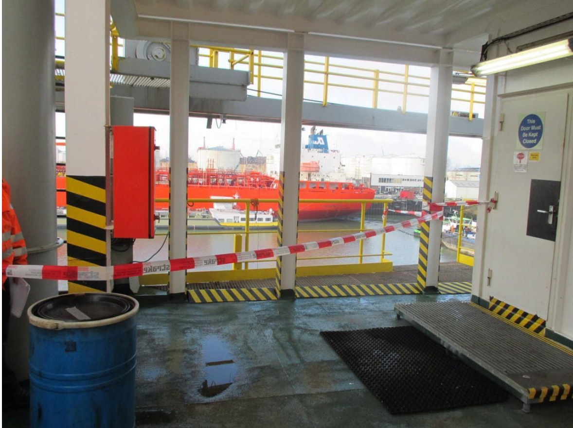
Figure 2 - Working space barricaded with red/white barrier tape
