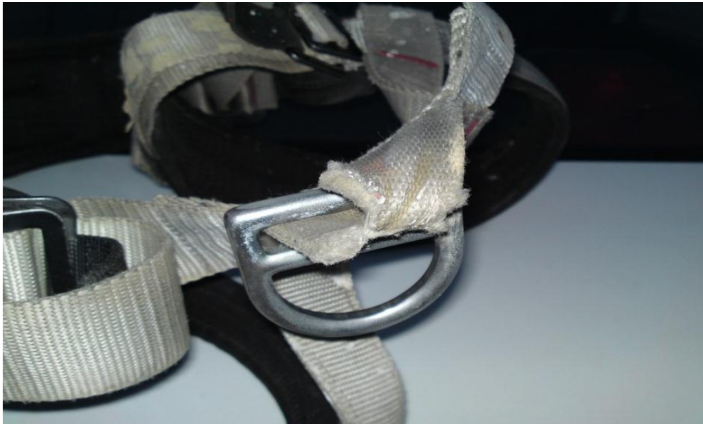
Excessive wear on webbing loop of a sit harness
